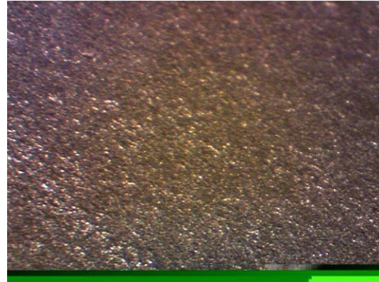
Fig. 5a Picture of void test of solder joint encapsulant paste
