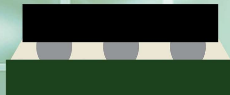
SMT 160 is a void free underfill and exhibits no slump when printed
