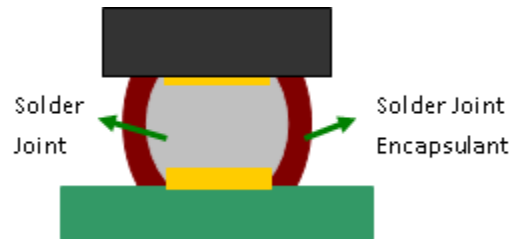
Figure 2. Schematic Cure SMT256 or SMT266 Encapsulated Solder Joint
