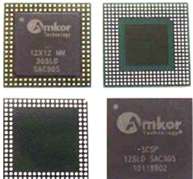
Figure 3. Amkor POP test Coupon
