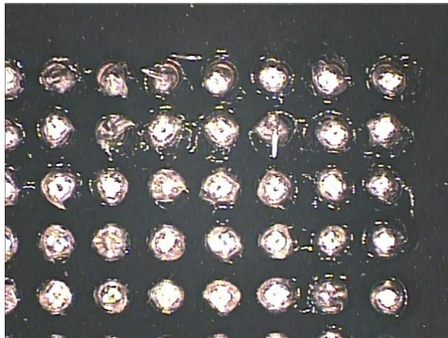
**Figure 14. Substrate after BGA Removal**
