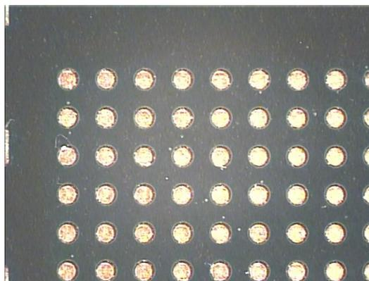
**Figure 15. Substrate After Rework**
